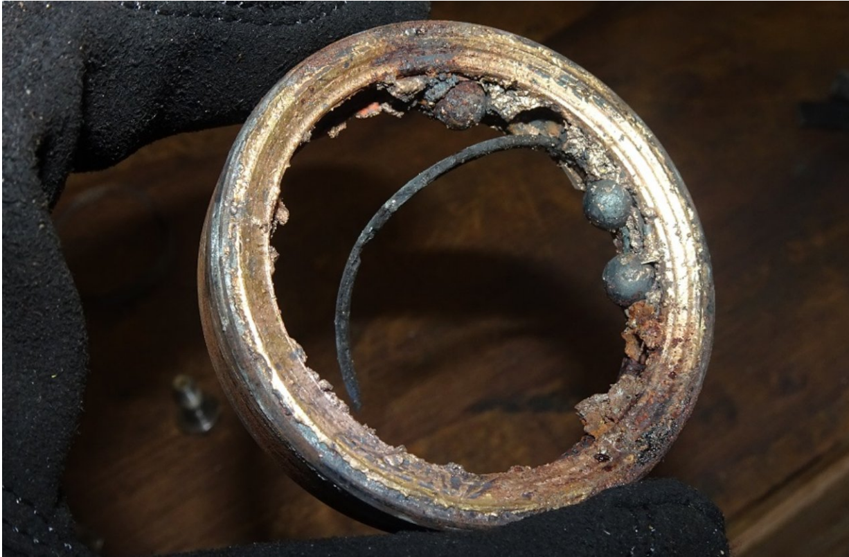
Figure 2. The clutch output bearing outer race with the three roller elements adhered.
