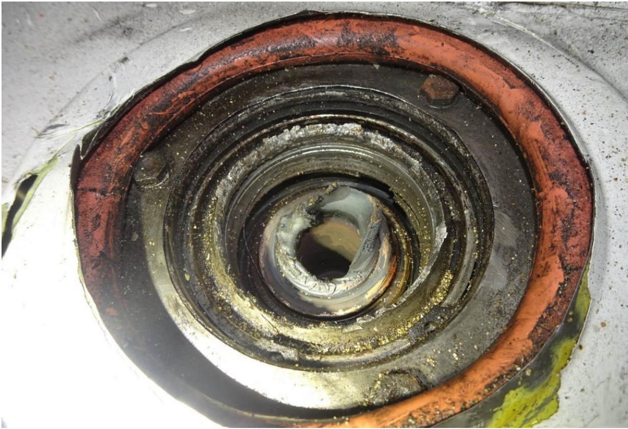
Figure 1. The fractured and thermally deformed clutch inner race.
