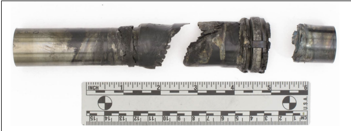
Figure 3. Turbine-to-compressor coupling shaft fractured. Photo courtesy Rolls-Royce.
