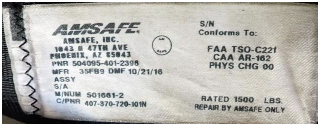
Figure 4 Example label marking of restraint that does not meet TSO-C114 or TSO-C22g requirements
