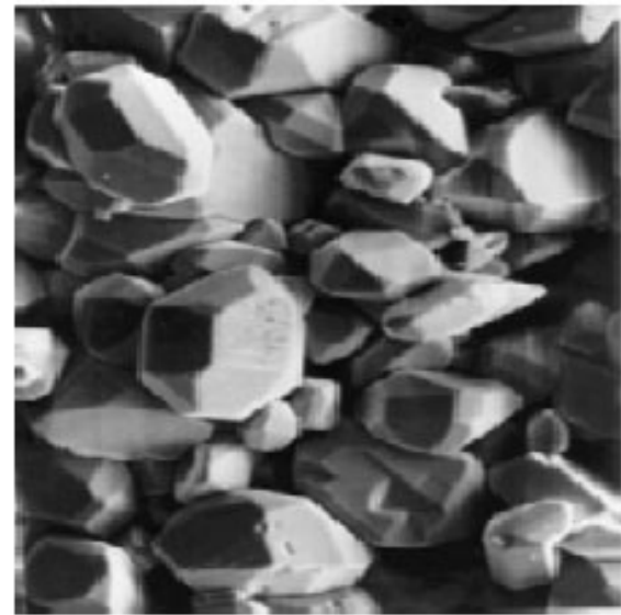
Hardening Lead Sulfate Crystals
