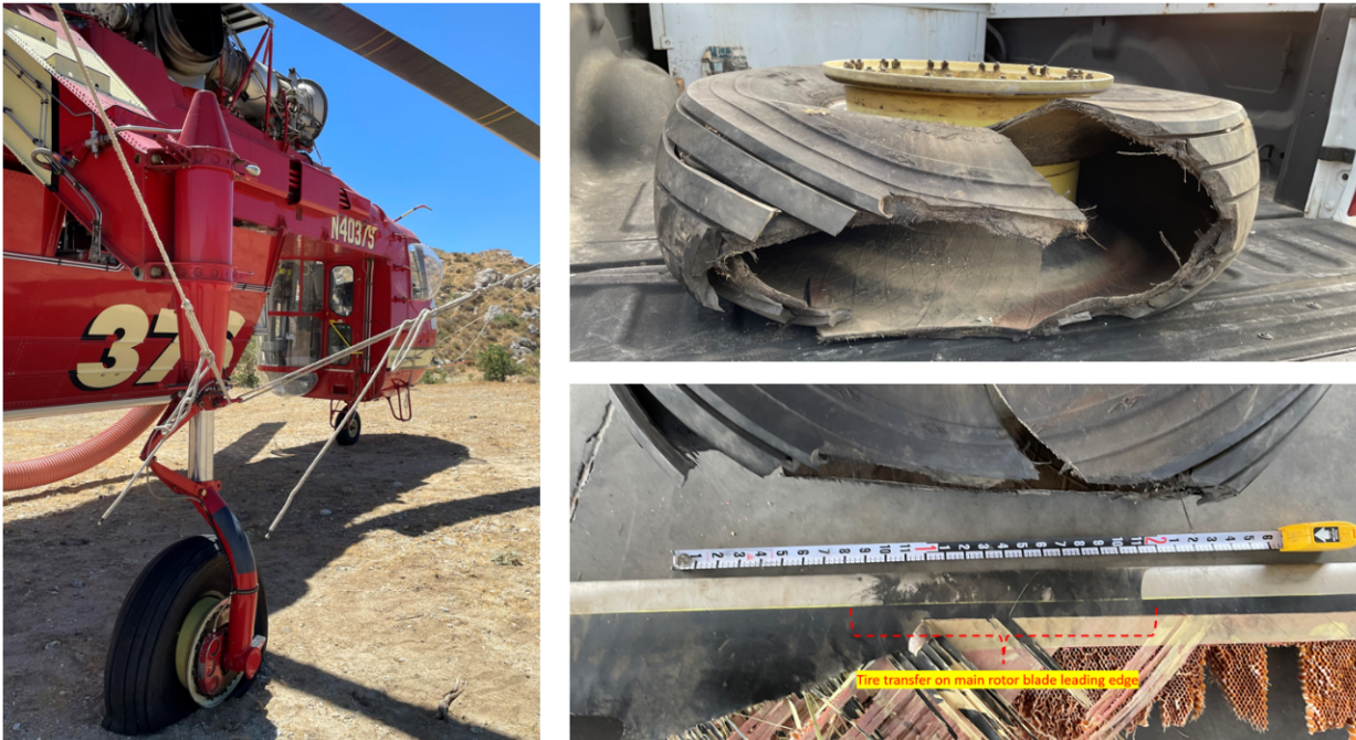
Figure 3. Left photo - view of damaged tire on helicopter. Upper right photo - view of removed damaged tire. Lower right photo - view of damaged tire next to main rotor blade showing transfer mark.
