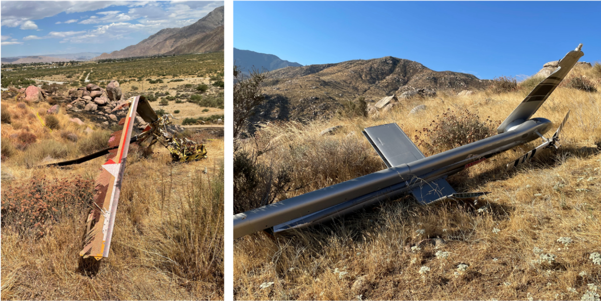
Figure 6. Left photo - view of main rotor and transmission assembly. Right photo - view of separated tail boom.
