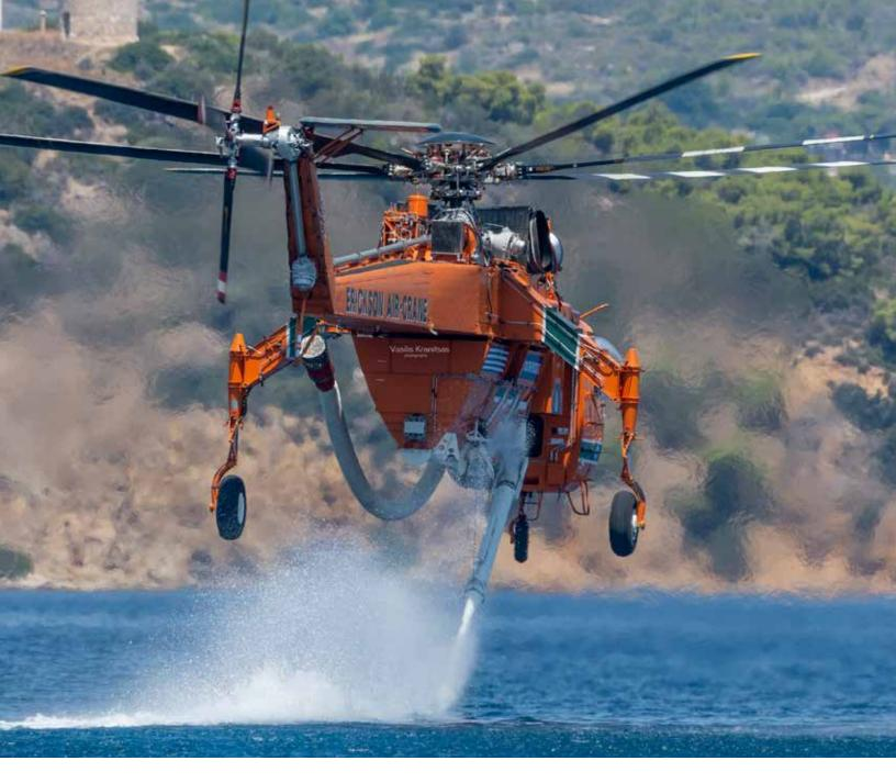
Air Cranes, like the one shown here in Greece in July 2020, are used to fight wildland fires on five continents. The aircraft's 25,000-lb. payload, coupled with its ability to refill water tanks in one minute or less, makes it an effective firefighting tool.
