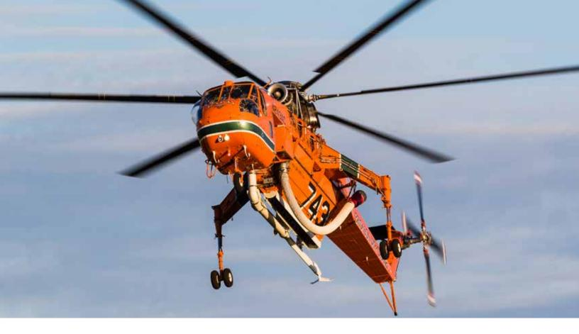
A partial list of mission-specific equipment that can be added to an S-64 includes hoists, a fire tank, a foam cannon, a grapple, and a sea or pond snorkel.
