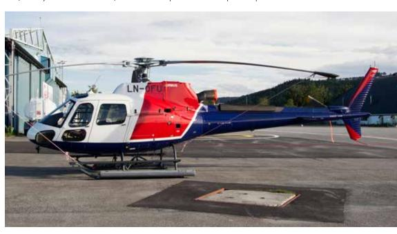
right and pitch up while the flight controls seem to have locked. While the AS350 flight manual describes this condition as "self-correcting," it can cause significant altitude and attitude excursions unless the pilot can compensate with muscle power or promptly reduce the loading.
