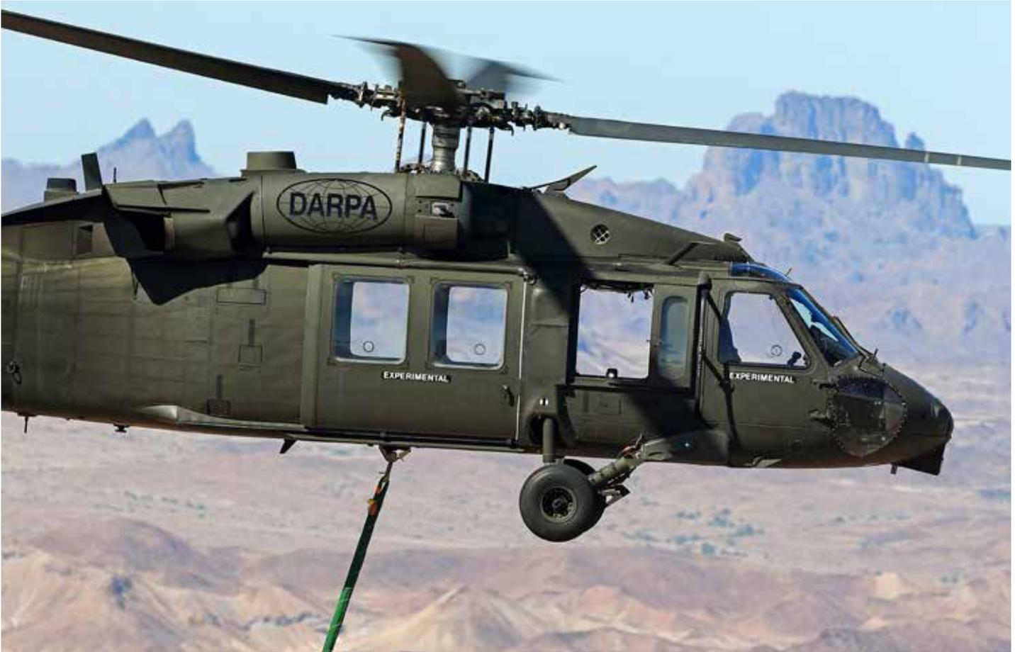
In 2022, an unmanned Black Hawk equipped with Sikorsky's Matrix autonomy technology flew as part of a US DARPA demonstration project in Arizona.
