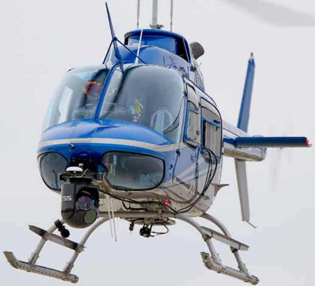
Shadowed by a drone capturing the action, a Bell 206B-3 operated by A&P Helicopters (also a VAI member) flies a Gyro-Stabilized Systems S512 five-axis aerial surveillance gimbal while flight testing new mapping features. The system includes 4K optical and high-definition mid-wave infrared sensors with a laser range finder, supported by software for object tracking, augmented reality map integration, and navigation.
