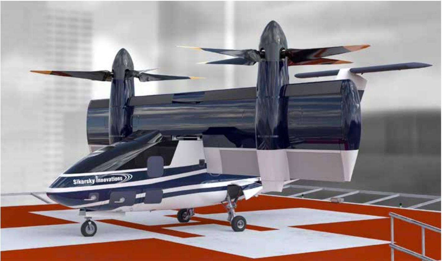
The HEX aircraft platform features a tilting wing, as opposed to tilting rotors and/or nacelles.
