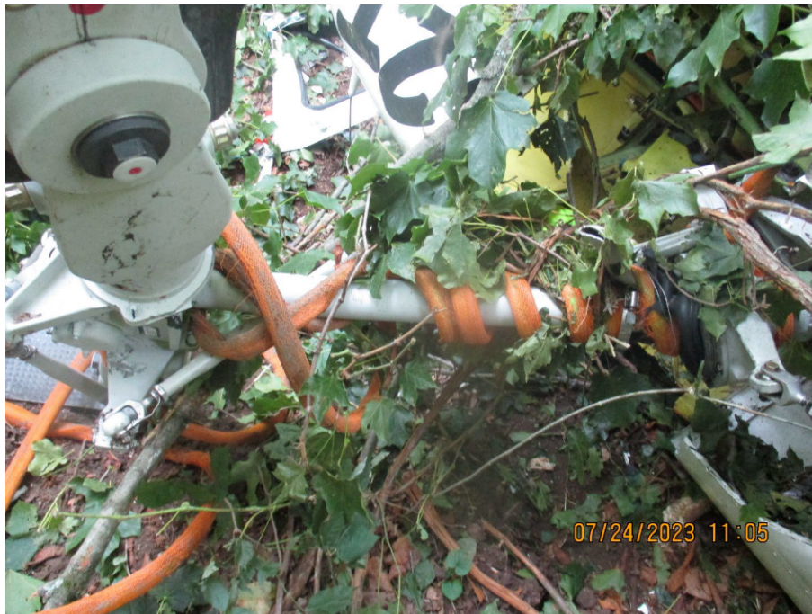
Figure 2. Long line wrapped around the helicopter main rotor driveshaft at the accident site. (Source: FAA)
