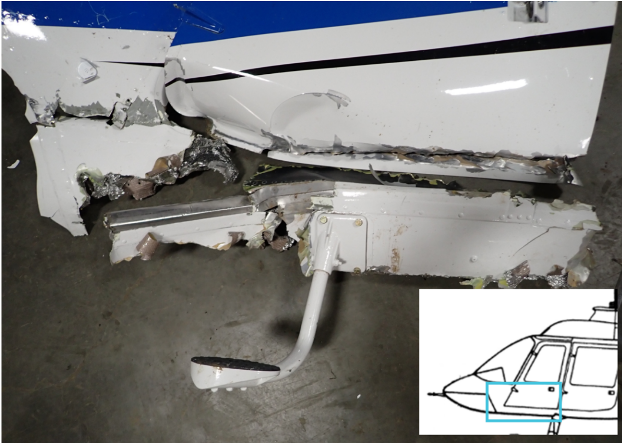
Figure 3: Tearing on the lower left fuselage. The inset depicts the area of damage on a model, with the damage area shown in the blue box.
