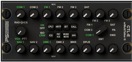
HEMS configurations consist of dual CTL-E control heads for pilot & flight nurse operations allowing for independent functionality during critical medical flight missions.
