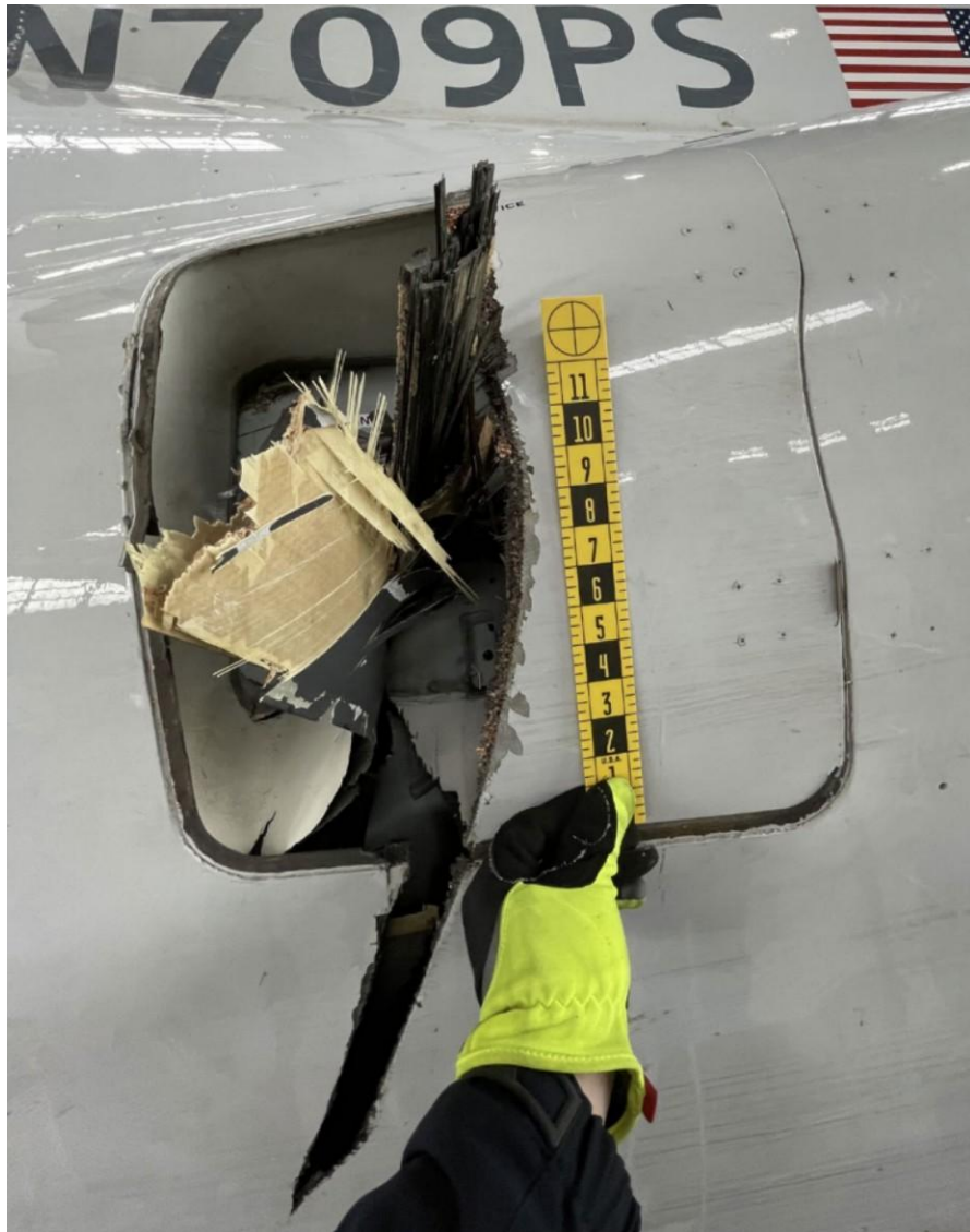
Figure 5. Damage to aft fuselage with tail rotor blade.
