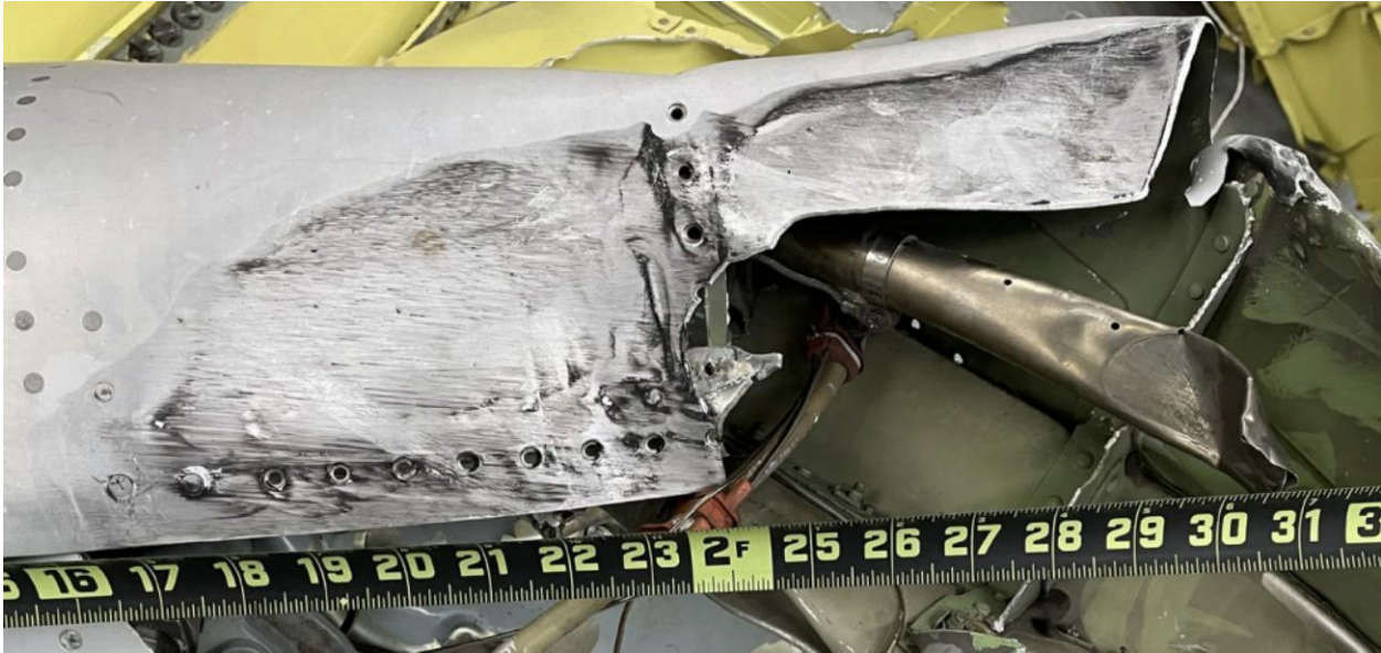
Figure 7. Close up view of impact mark on left inboard slat.
