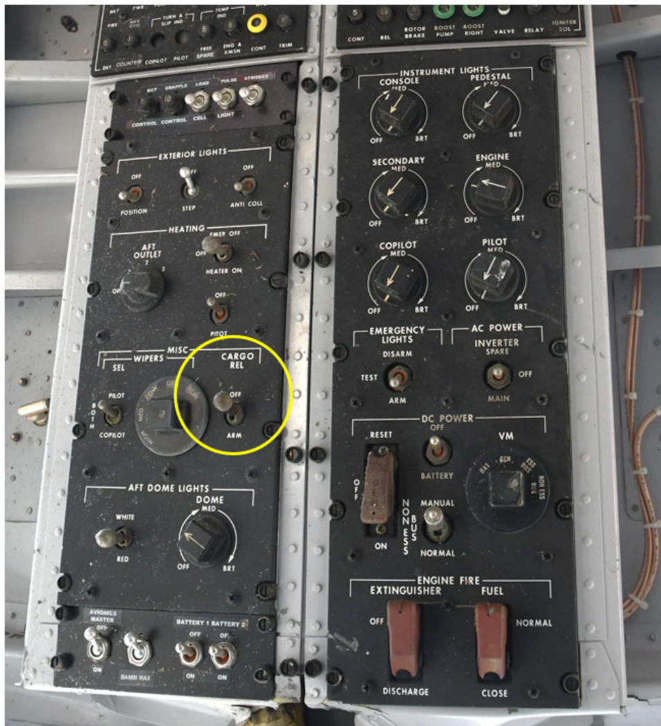
Figure 11. CARGO REL [cargo release] switch, as found post-accident, on the overhead panel of the occurrence helicopter. DC Power and Battery switches were selected OFF, post-accident, for safety reasons. (Source: TSB)
