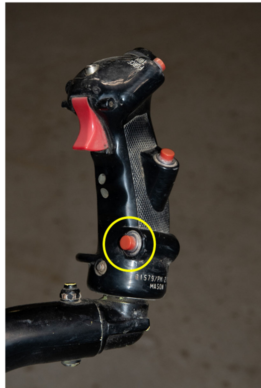
Figure 10. Electric cargo release push button on the cyclic from the occurrence aircraft (Source: TSB)
