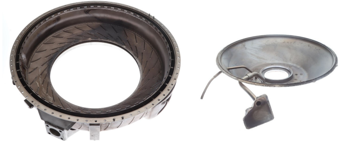
Figure 5. Air diffuser casing assembly (left) and No. 2 bearing support cone (right) separated at the braze joint (Source: TSB)
