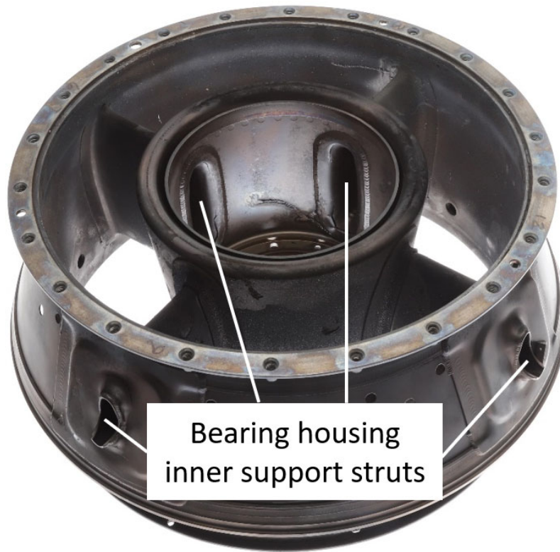
Figure 7. Exhaust diffuser showing the bearing housing inner support struts (Source: TSB)
