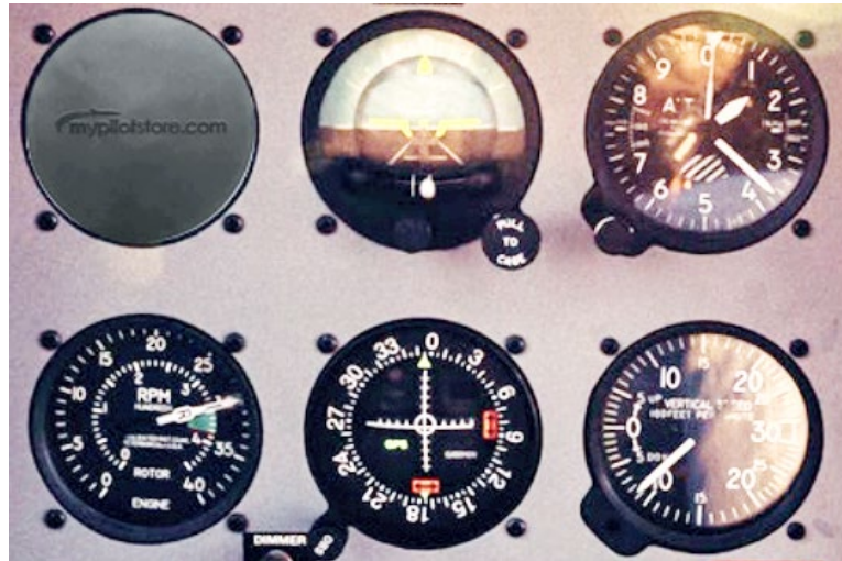
Figure 23 Limited/Partial instrument panel with failed ASI covered[10]
