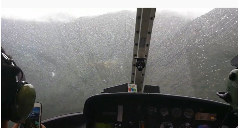
Figure 4 Example of marginal and deteriorating VMC
