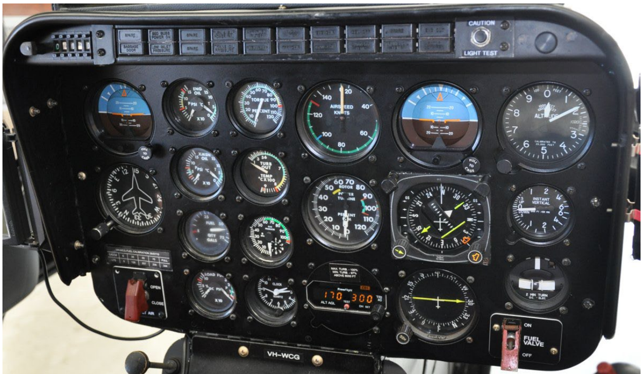
Figure 22 Instrument panel with analog instruments with a standby AH and DG
