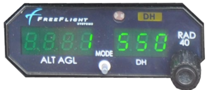
Figure 32 Digital radar altimeter
