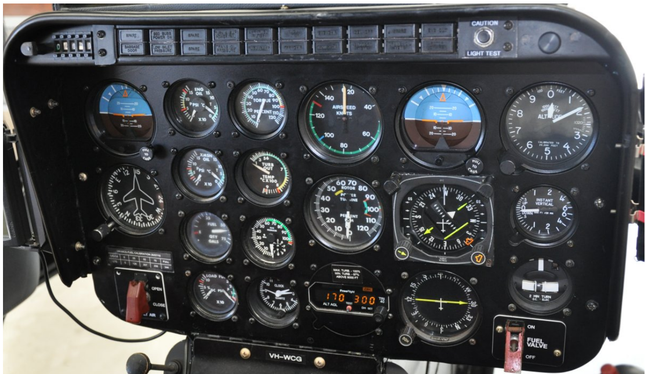
Figure 16 Instrument panel with analog instruments with a standby AH and DG
