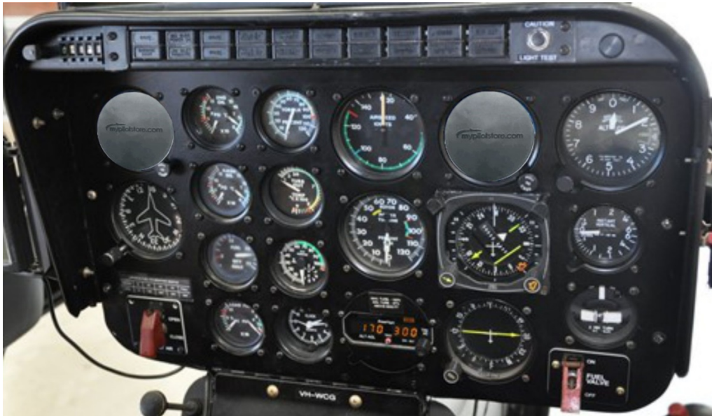
Figure 17 Limited/Partial instrument panel with failed ASI covered
