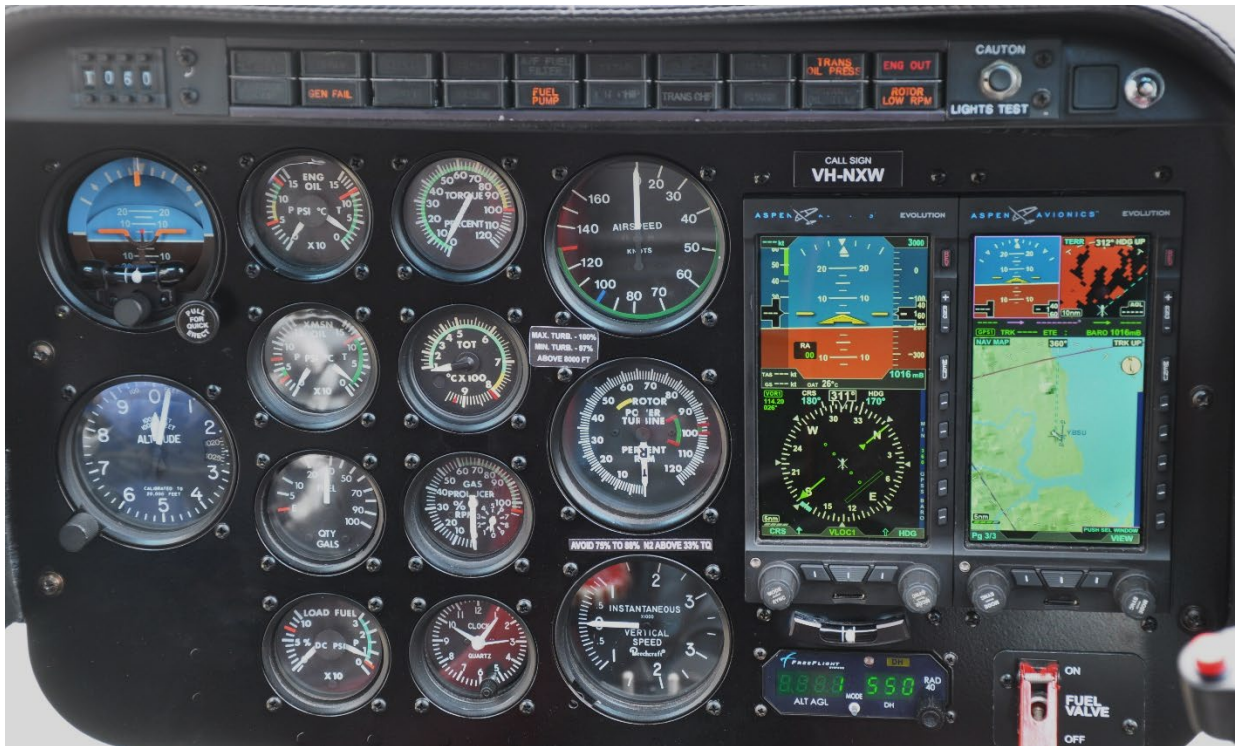
Figure 18 Instrument panel showing a digital (Aspen) glass cockpit with a standby AH and altimeter
