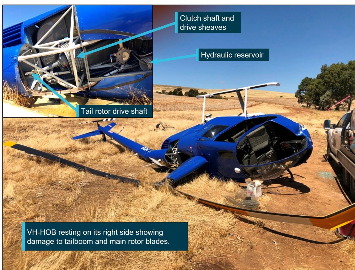
Figure 2: VH-HOB following the collision with inset showing clutch shaft with upper drive sheaves and displaced hydraulic reservoir
