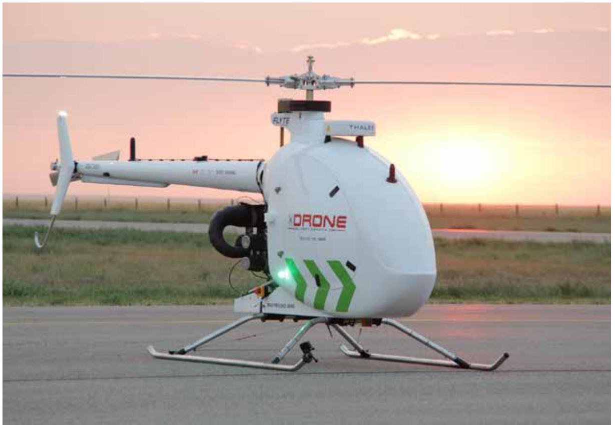
The 1,050-lb., gasoline-powered Condor drone can carry a payload of 400 lb. 125 miles at 75 miles per hour on preprogrammed routes to specific drone spots.
