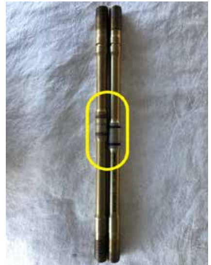
The part on the right (above) was improperly engineered, with its center dowel section out of position.
