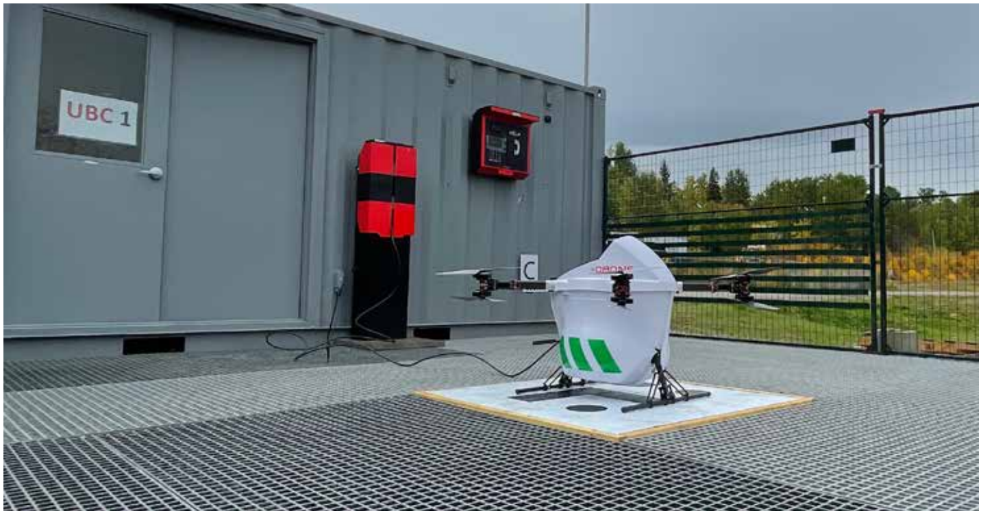
The Sparrow battery-powered drone operates on preprogrammed routes to and from drone spots such as this fenced-in area. It can carry up to 9-lb. payloads at speeds up to 50 miles per hour. The company's logistics system tracks all packages. A Sparrow is now operating on a short route from Edmonton International Airport (CYEG).
