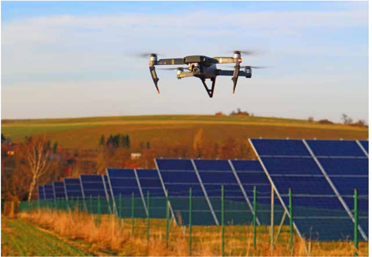
Engineers use a DJI Mavic Pro drone to inspect solar panels near Pilsen, Czech Republic.
