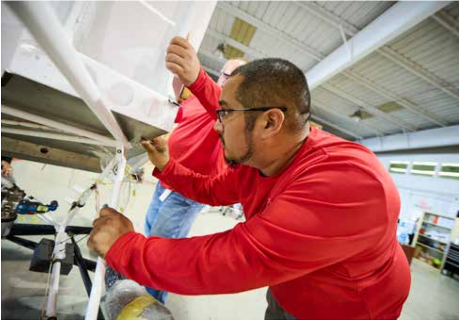
Andrew Granado oversees the precision placement of a cabin on a fuselage. Schweizer worked closely with the FAA to set up and certify the plant's manufacturing line.
