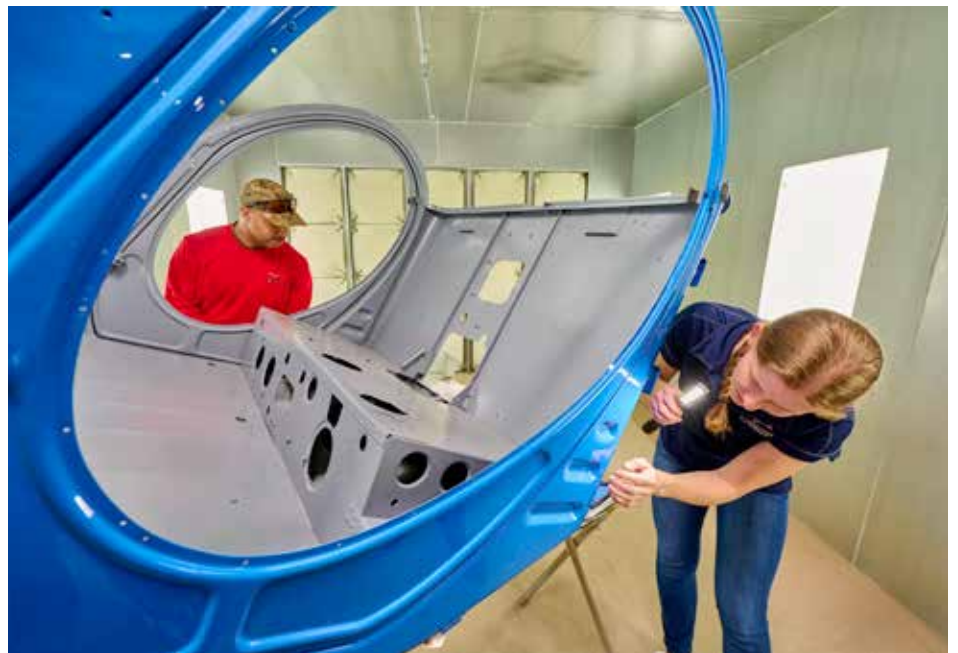
Angie Thornton performs the final visual surface inspection of a painted cabin, ensuring it meets required standards.
