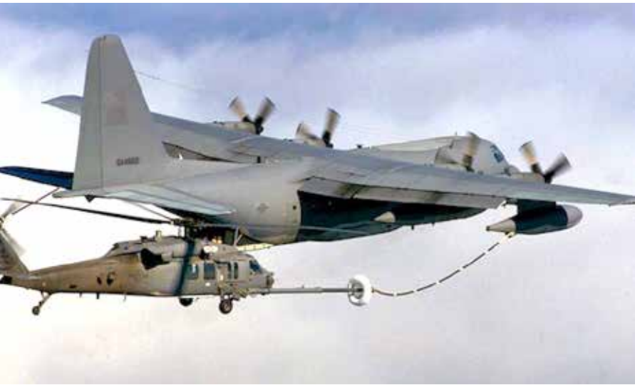
An HC-130 Combat Shadow refuels an HH-60 Pave Hawk. Midair refueling requires precision flying by both pilots, even in daylight and good weather conditions.
