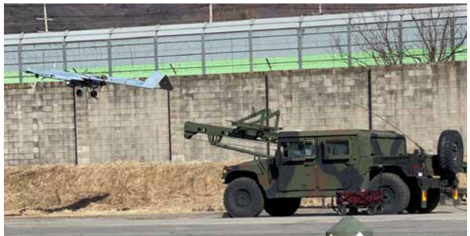
A team from the Army's 1st Infantry Division launches the Shadow, the unit's unmanned aircraft. The drone appears almost airplane-like, given that it weighs approximately 450 lb. and has a wingspan of nearly 25 ft.
