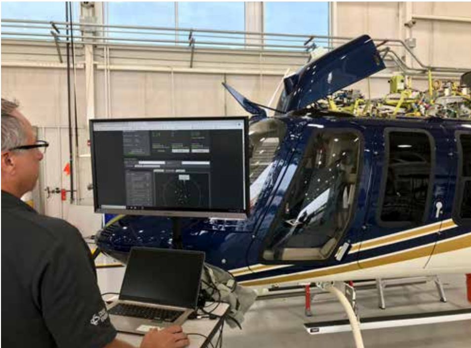
A technician consults the Foresight dashboard for this Bell 407GX; see the opposite page for a closer look at the types of data available through Foresight.
