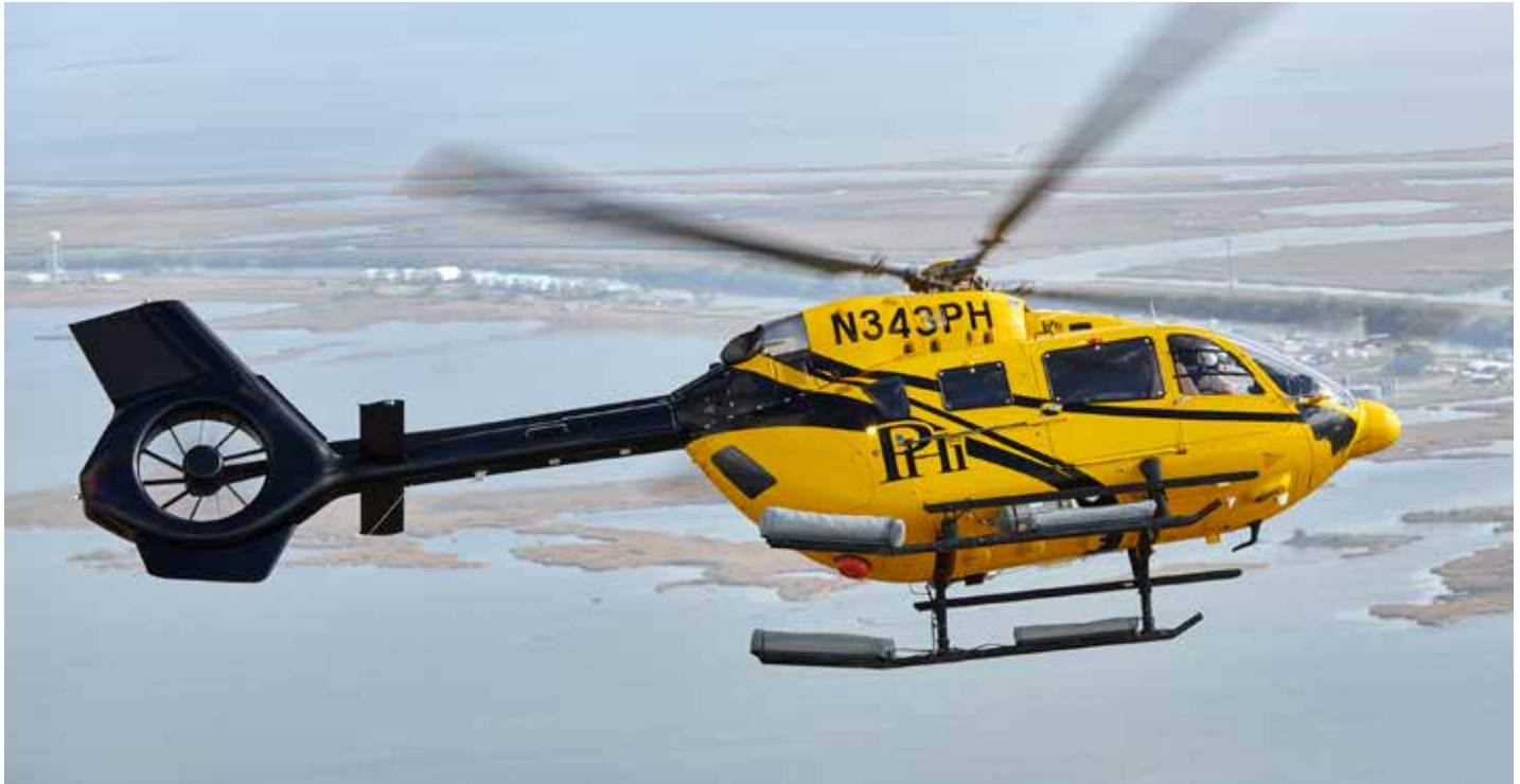
Above: The most obvious difference between the H145 and an earlier model, the EC145, is the Fenestron tail rotor, which reduces noise and improves safety.
