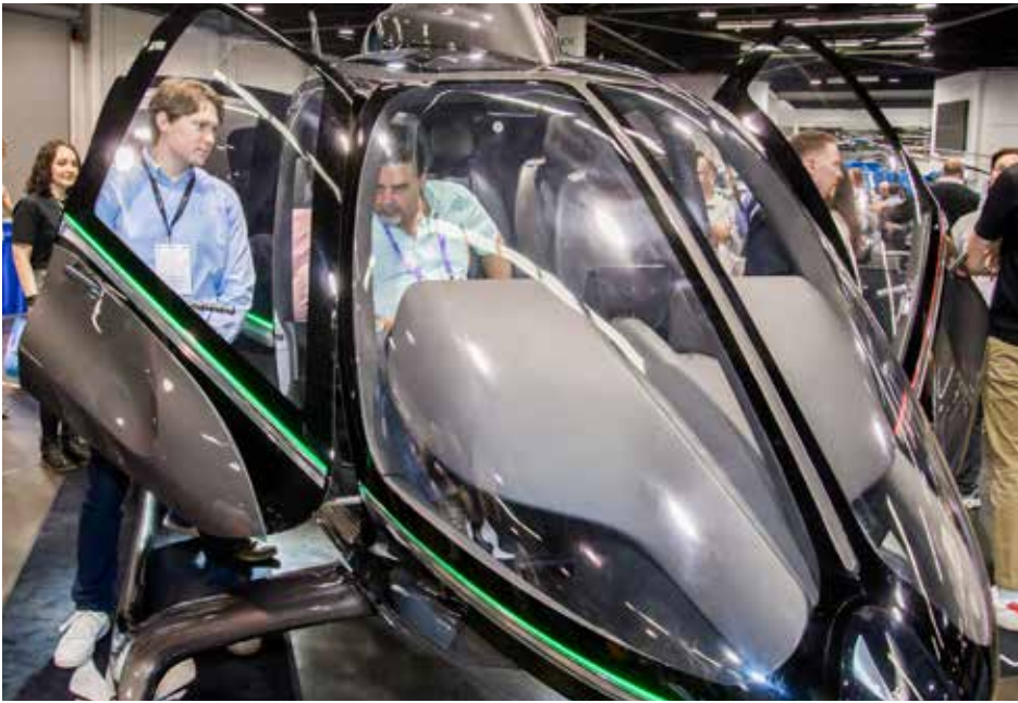
Hill Helicopters' HX50 model is a clean-sheet design still in development. It promises a range of 700 nm, cruise speed of 140 kt., payload of 1,760 lb., and styling on a par with luxury automobiles—all at a base price of about $756,000.
