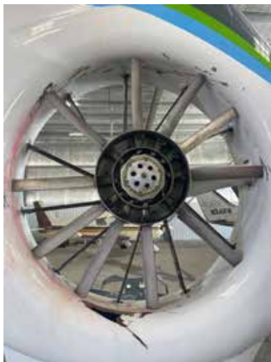
An Airbus EC135 P2+ sustained substantial damage to its Fenestron assembly when a cover was blown off of a fire extinguisher and ingested into the tail rotor. The entire tail boom had to be replaced. (NTSB Photo)
