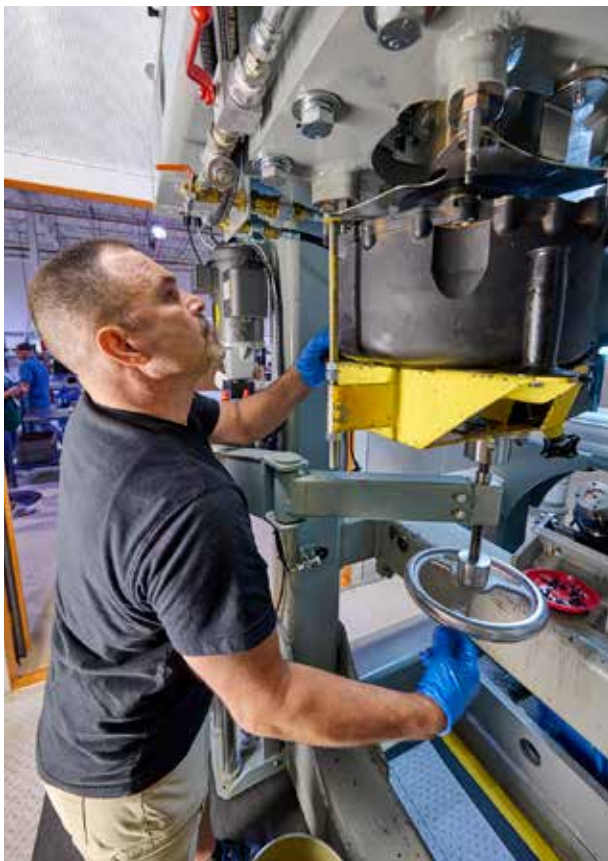
Level 5 mechanic Mike Gayler installs a main-rotor transmission into the test cell in the company’s aftermarket operations center.
