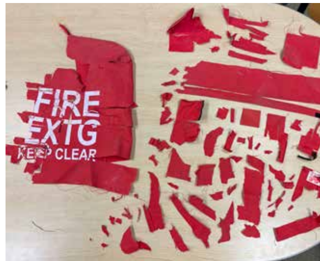
An Airbus EC135 P2+ sustained substantial damage to its Fenestron assembly when a cover was blown off of a fire extinguisher and ingested into the tail rotor. The entire tail boom had to be replaced. (NTSB Photo)
